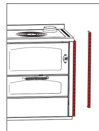
STAINLESS STEEL PERFORATED FRONT SIDE SPACER to fix on the side of the wood cooker. The customer's piece of kitchen furniture will have to be made with a top that is 25mm longer, as to cover the side spacer.
