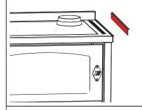
Since stainless steel has a high heat conductivity, should the customer's top of the kitchen furniture not be made out of stone or similar materials, we advise to always place a STAINLESS STEEL PROFILE between the top of the kitchen furniture and the wood cooker top.
