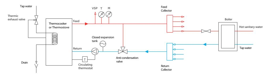
M= Manometer VSP= Over-pressure valve T= Thermometer
